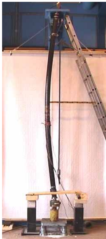
Fig. 6: Specimen C3600 after buckling.
