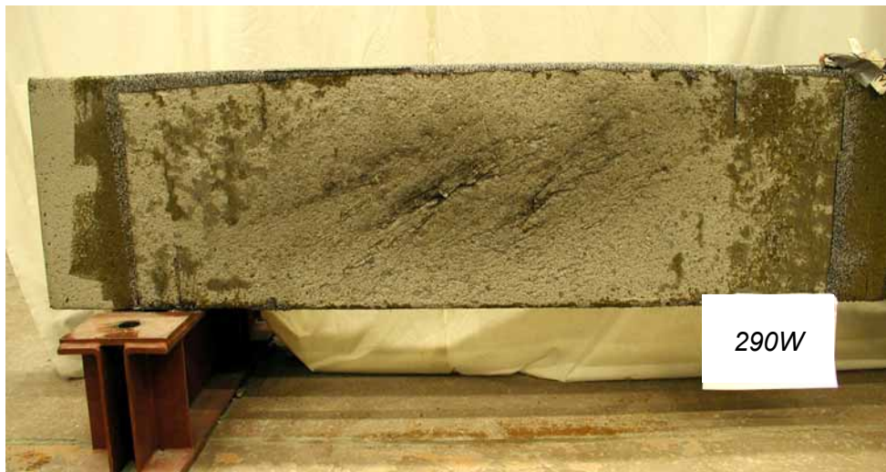
Fig. 14. Crack zone before ultimate shear failure
